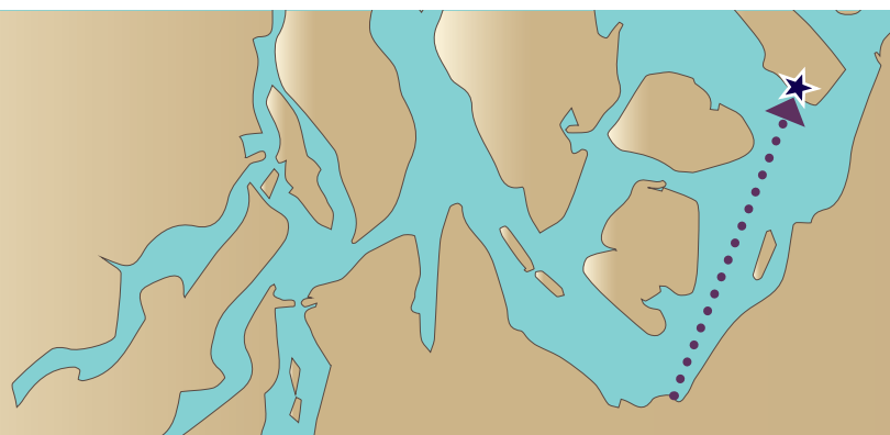
Maximum fetch (arrow) is the longest distance across open water to a site (star).
